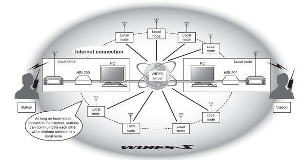
With the WIRES-X system, voice communication is carried out in the following manner:
