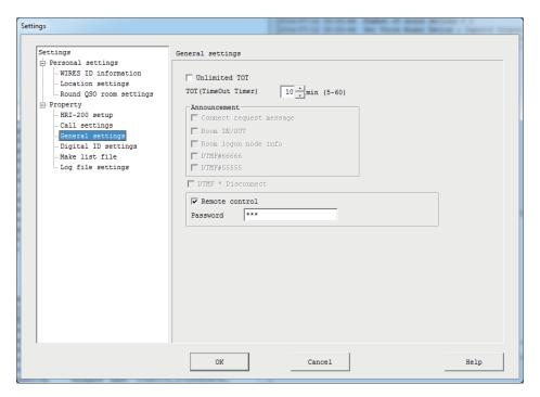
Unlimited TOT.....Set whether or not to limit the connect time by activating the timeout timer (TOT) when your node is connected to a node or room.
