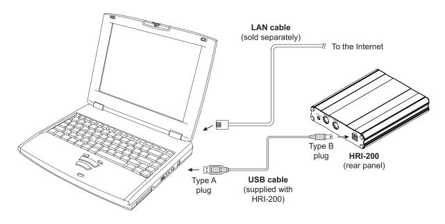
When the HRI-200 is connected to the PC properly, the HRI-200 will turn on automatically when the PC is turned on.
